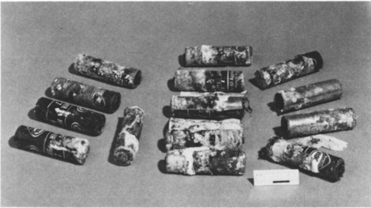
Fig. 22. HP7 zinc—carbon batteries. All were charged when buried. Most have the outer plastic wrapper removed to reveal corrosion of the zinc cans.
