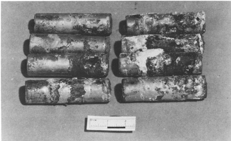
Fig. 24. HP7 Zinc—carbon batteries. For comparison the left hand batteries were charged and the right hand batteries discharged when buried. The white 'furry' deposits formed on standing in the laboratory.
