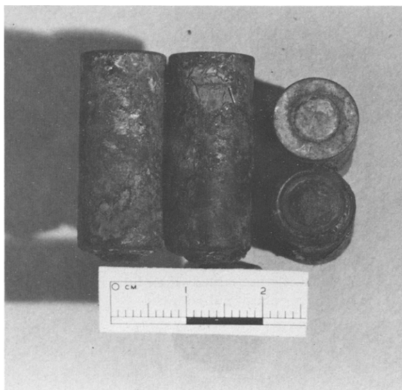
Fig. 16. RM401 mercury batteries. The left hand cell was charged and the others discharged when buried. The second cell from the left was damaged during the excavation.
