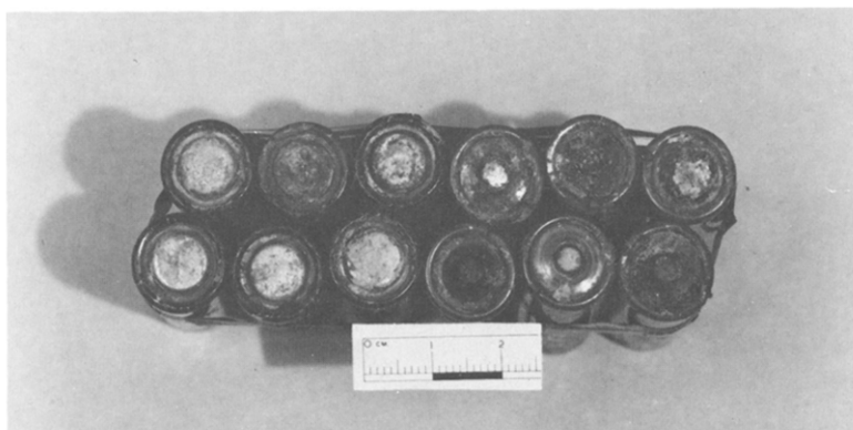
Fig. 15. MN1500 alkaline—manganese batteries. For comparison the top row were charged and the bottom row discharged when buried. The negative terminal buttons (left) were largely unattacked while the positive terminal buttons of the charged batteries (top left) were substantially attacked.
