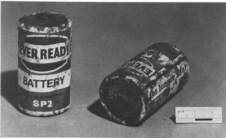
Fig. 21. SP2 zinc—carbon batteries. Discharged when buried.
